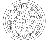
ME connector (32 pin) Glenair IPT 02 A 18-32 P F6 front view
