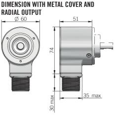
recommended mating shaft tolerance H7 dimensions in mm
